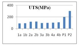
Fig. 9 Ultimate Tensile strength of parent materials and weld joints.
