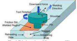
Fig. 1 Friction stir welding process [2]
