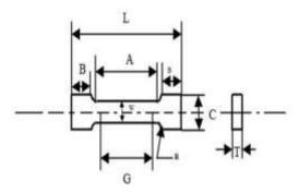
Fig. 6 Tensile test specimen diagram
