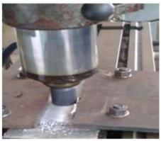
Fig. 4 FSW experimental Set-up
